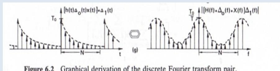
Figure 6.2 Graphical derivation of the discrete Fourier transform pair.
